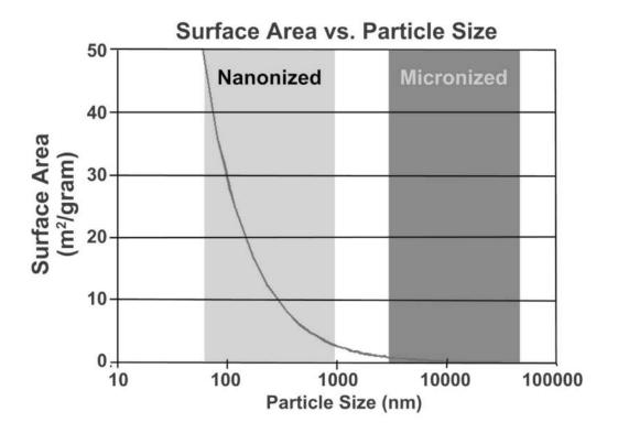
Figure 1: The plot demonstrates the increase in surface area obtained when solids are fractured from the micron-size range (microparticles) to the nanometersize particles used in the various nanoparticle formulations to improve the performance of poorly water-soluble compounds (Cortesy: Elan Drug Technologies)
